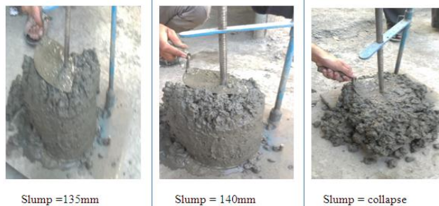
Figure no. 1 “slump test on fresh concrete”
